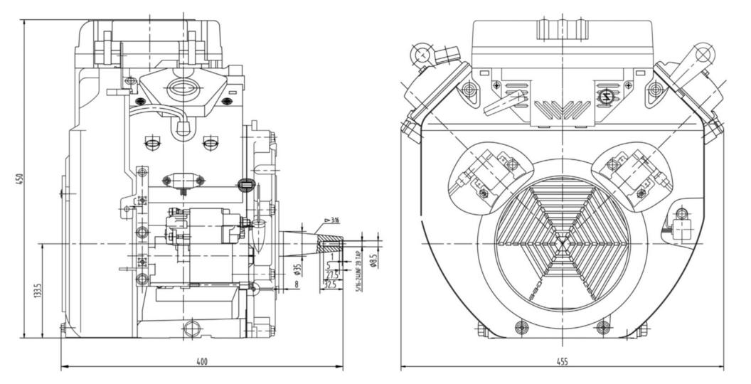
24HP V-TWIN - Mounting & Measurements
