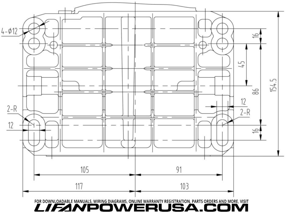
24HP V-TWIN - Mounting & Measurements
